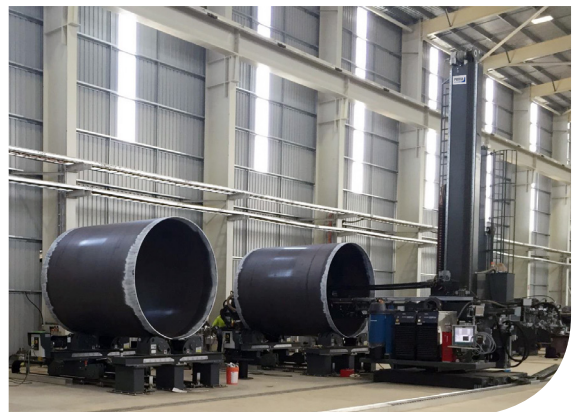
Longitudinal welding carried out by means of a C&B and PEMA N rollerbed stations.
