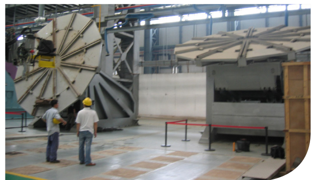
PEMA positioners commissioned at a customer site.
